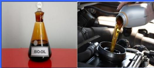
It is the conversion of biomass to liquid, (bio-oil or bio-crude), solid and gaseous state, by heating the biomass in the absence of air. This bio-oil can be used in engines and turbines.
